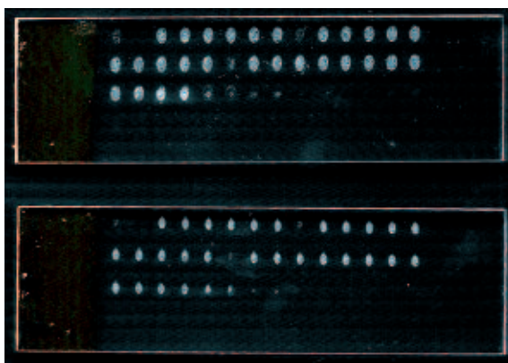
Figure 4. Image of used plasma mirrors; the first plasma mirror is shown in the top half of the image (ellipse spot size 2 \times 3 mm) and the second plasma mirror is in the bottom half (ellipse size 1 \times 2 mm).
