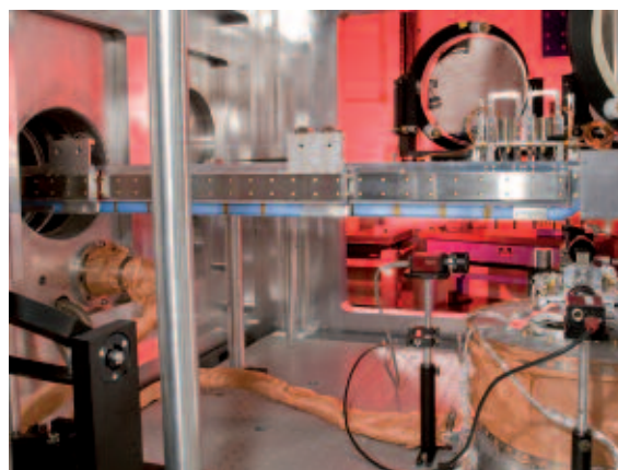
Figure 2. Target Inserter arm extending into the Astra Gemini interaction chamber to retrieve a target puck.
