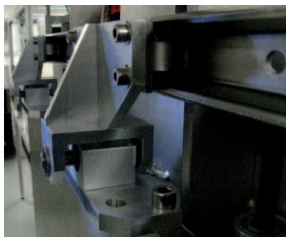
Figure 1. New door mechanism on the Gemini North compressor.
