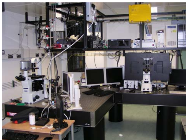
Figure 8. Left: TIRF-Tweezers set up. Right: One-photon confocal.
