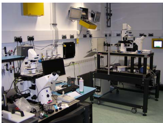
Figure 5. Left: Experimental setup for 3-colour single molecule tracking system. Right: experimental setup for multidimensional single molecule fluorescence imaging. The picture shows a wall-mounted black panel between the microscopes below the open yellow box on the wall. This black box houses the array of fibre connectors that allow laser light to be transported via fibres, combiners etc. from the adjacent laser hub in the OCTOPUS core to the microscope room through the wall. These boxes can
