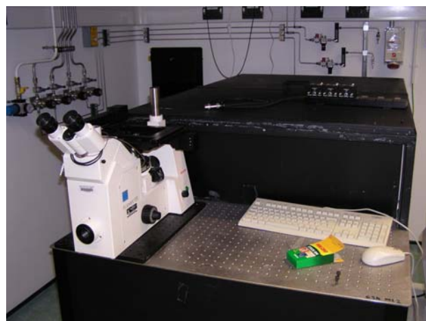
Figure 7. One-photon multicolour confocal system. In-house built confocal microscope that uses a Fianium supercontinuum as laser input.
