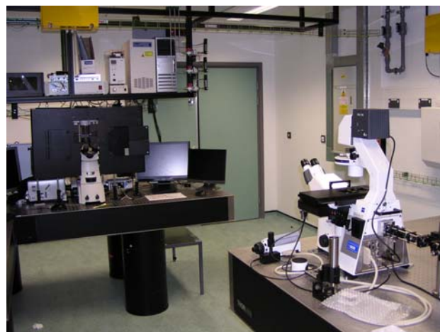
Figure 6. Left hand side: one-photon confocal FLIM system. Right hand side: 5-colour single molecule fluorescence microscope.
