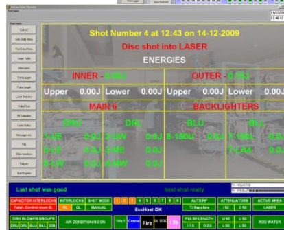
Figure 1b - Main control screen giving access to prime control functions and diagnostic data such as the shot firing sequence and waveform displays.
