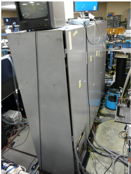
Figure 2 – Old Quantel rod amplifier racks inside Laser Area 1 that charged the 16mm and 25mm amplifiers.
