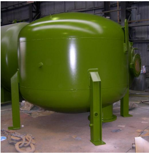
Figure 6- showing an example of an air receiver.
