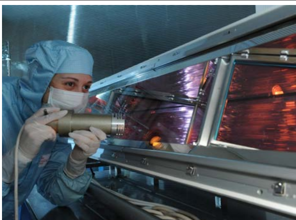
Figure 1: Inspection of 150 Rectangular slab amplifier
