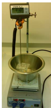
Fig. 8: Silicon wet etching with KOH at 80 C.
