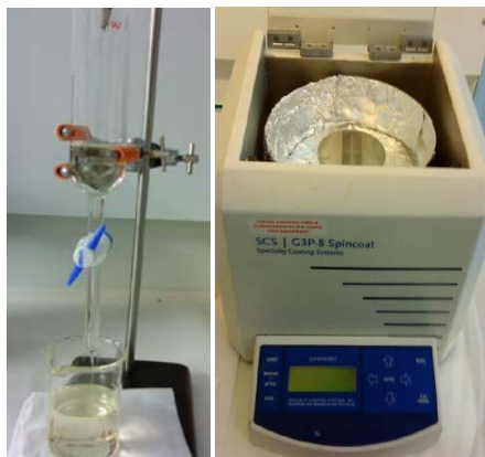
Fig. 5: Glass cylinder for dip coating (left image). Spin coater (right image).
