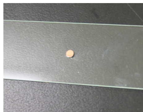
Figure 2b: The original setup of a 25µm Cu aperture glued on top of a microscope slide.
