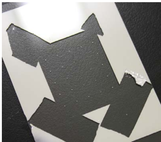
Figure 4(a) shows a microscope slide after being coated with aluminium through the 100 micrometer diameter copper pinhole array.
