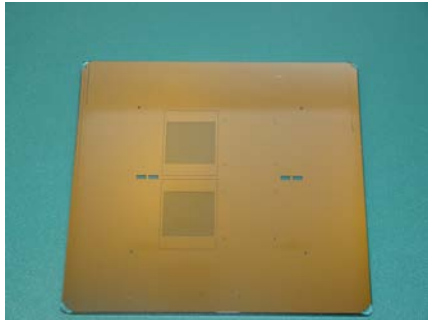
Figure 1. CAD design for the Fe dot target photomask (top) and photograph of the finished photomask (bottom).
