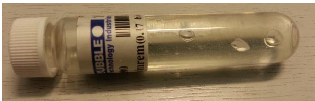
Fig.1 A single bubble detector tube with visible bubbles
