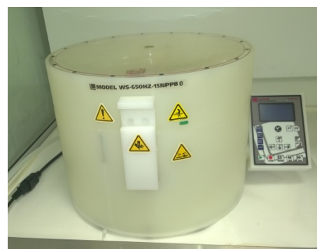
Fig. 5: Large area spin coater for (thin) film production
