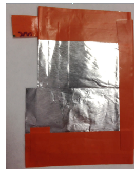
Fig. 2 Filter pack used to create 10 zones of filtration each layer is 26 \mu m thick Aluminium foil.
