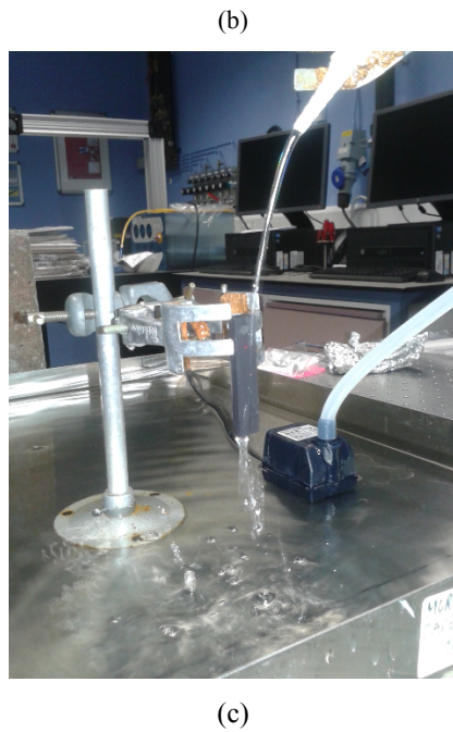
Figure 1 Set-up of the LSP technique in (a); and (b and c) showing the optical images of the LSP of \text{Si}_3\text{N}_4 at 80% coverage and 50% overlap.
