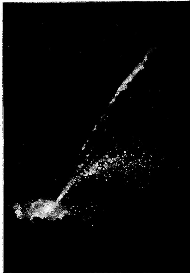
Figure 4.06 Parabola obtained from a target that was nominally pure gold. Again hydrocarbon contamination can be seen.
