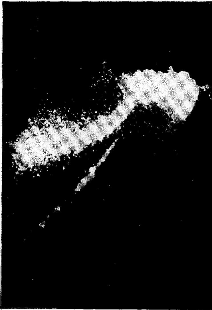
Figure 4.05 Parabola obtained from a vanadium target, showing a proton parabola. The carbon parabola are masked by the vanadium parabola.
