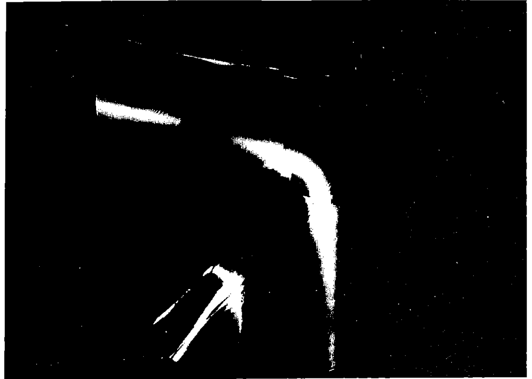
Fig A4.30 Schlieren image of the bow shock around an obstacle placed in plasma ablating from a source at the top right. The stalk supporting the obstacle is also visible
