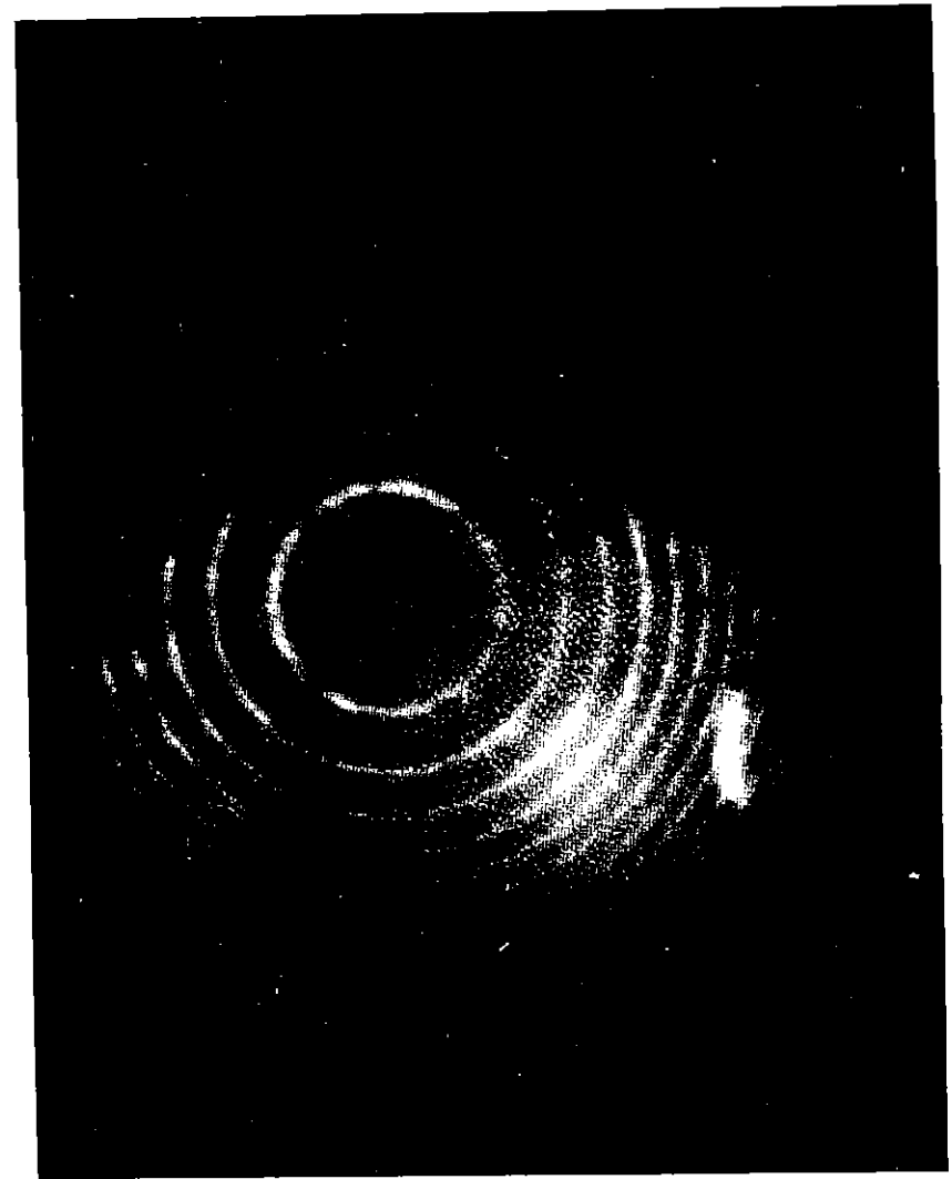
Fig B4.4 Fabry Perot interferogram of line-narrowed output of stabilised EMG 150 running at 10 Hz. Free spectral range of interferometer = 2 \text{ cm}^{-1} .
