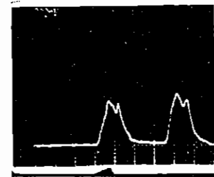
Typical input & output beams for the second amplification 10ns/div
