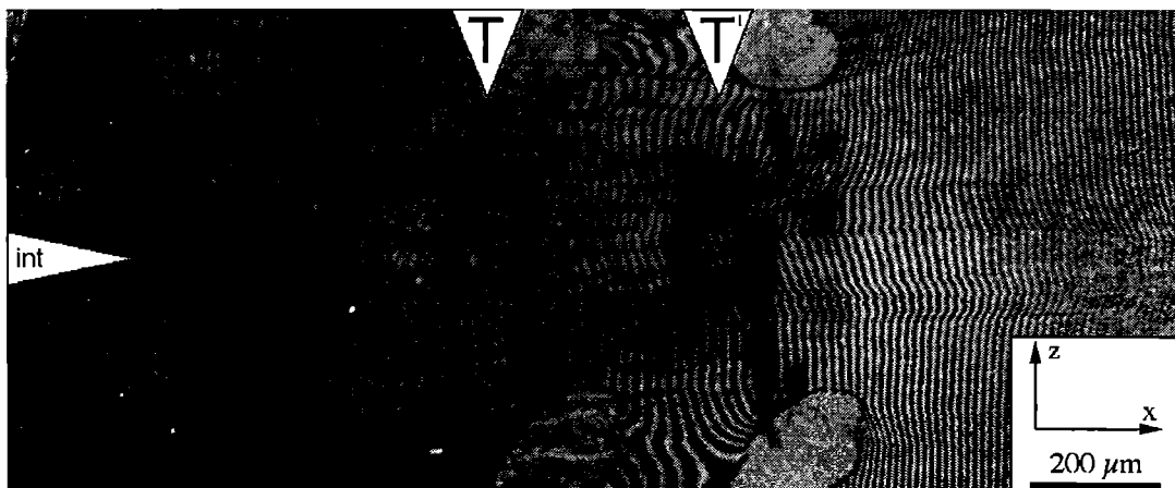
Fig. 4: interferogram of the plasma 300 ps after the interaction with the short pulse. The horizontal arrow shows the short pulse interaction axis. The vertical arrows show the original target position.
