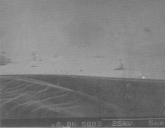
Fig. 1 SEM image of a 95 \pm 5 nm thick a-D film on Si(100) formed by PLD of a high density graphite rod for 20 mins using an ArF laser delivering 250 mJ pulses at 10 Hz repetition rate.
