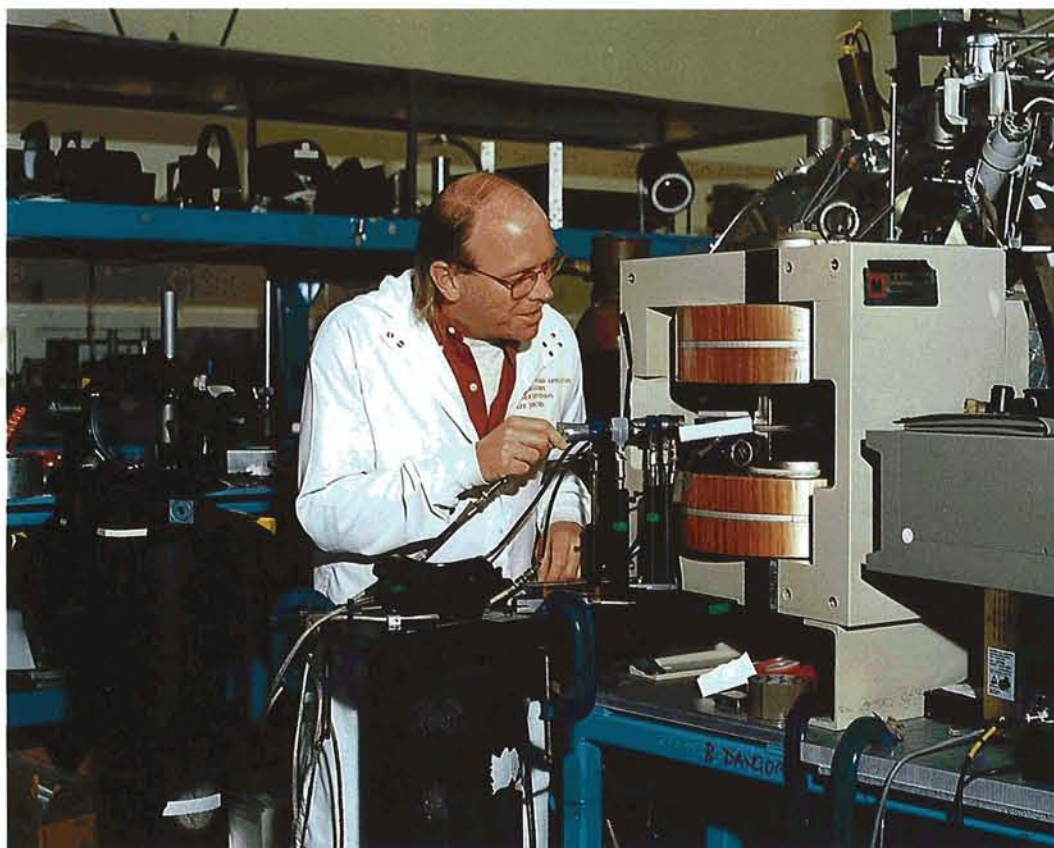
Chris Clayton of UCLA checks the alignment of the detectors in the electron spectrometer (96RC2662).
