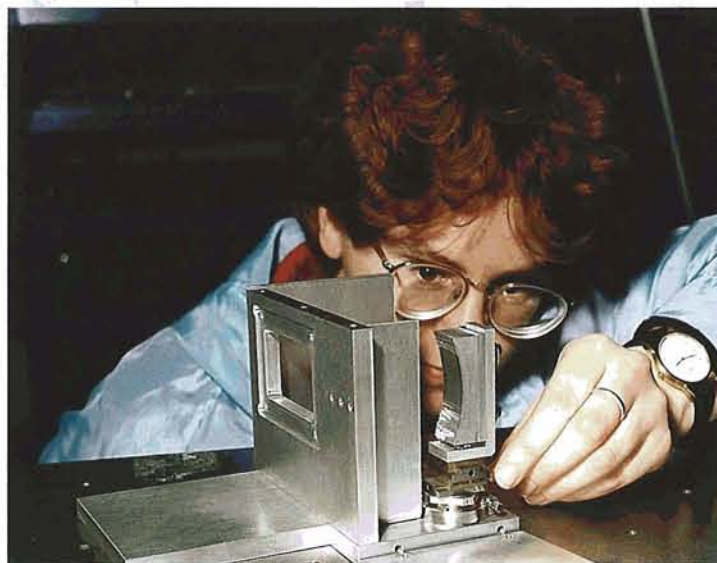
Margaret Notley of the Target Area Support Group adjusts a Von Hamos x-ray spectrometer designed to measure the density and temperature of a plasma (98RC1706).
