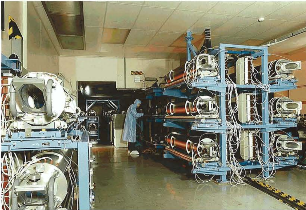
Placement student Steven Hawkes of Sheffield Hallam University aligning the output stages of Vulcan (97RC4284).
