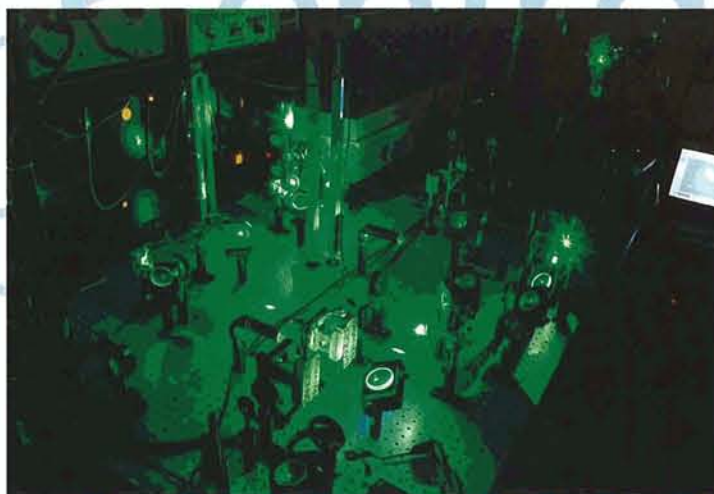
Testing of Vulcan's new broad bandwidth pre-amplifier based on the Optical Parametric Chirped Pulse Amplification (OPCPA) scheme developed within the CLF (98RC1697).
