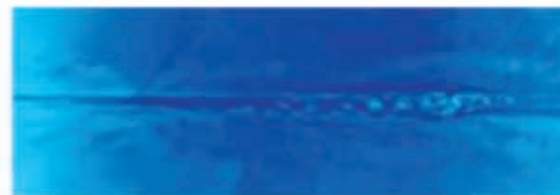
A proton projection image of the interaction of a high-intensity laser pulse with a jet of helium gas at 50bar pressure. The laser pulse propagates through the low-density plasma created by ionising the gas and undergoes a number of highly non-linear processes, including the excitation of large-amplitude electron plasma waves, the onset of relativistic channelling and filamentation, the generation of electromagnetic solitons. As an effect of these processes, complex plasma structures are formed in the wake of the pulse, which for the first time have been detected via the associated electrostatic fields using proton projection imaging techniques.
