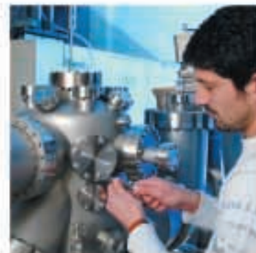
Dr Fred Jamme from the University of Nottingham attaching a blanking flange to the new ultra-high vacuum facility.
