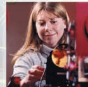
Peta Foster, CLF, optimising a parabola used in ultra high intensity experiments.
