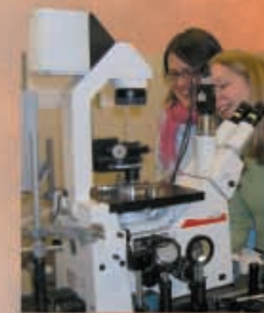
Rebecca Hopkins and Dr Laura Mitchem, University of Bristol, capturing aerosol droplets using the optical tweezers apparatus.
