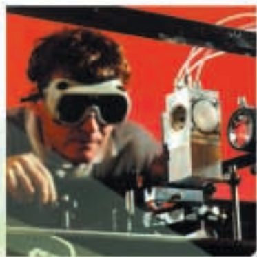
Dr Mike Towrie, CLF, aligning the ultrafast infrared spectrometer.
