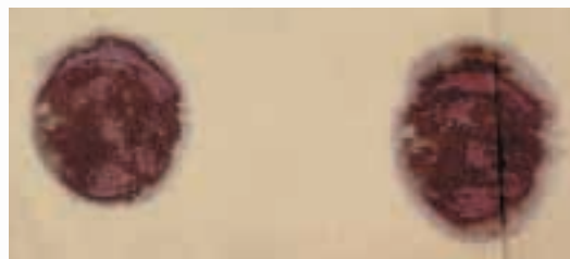
The two beams produced from the OPCPA amplification process, one of which is of high beam quality, which is subsequently compressed and sent to target, and the other which is of poorer quality and dumped
