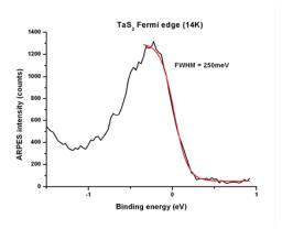
Figure 12. Measurement of the TaS<sub>2</sub> Fermi edge at 33.5 eV (photon energy37 nm).
