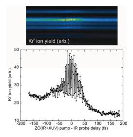
Figure 9. Zero-order (IR + XUV) pump, IR probe measurement, showing interference fringes between the two IR pulses. The asymmetry in the Kr+ yield is a consequence of the XUV also transmitted in the zero-order.
