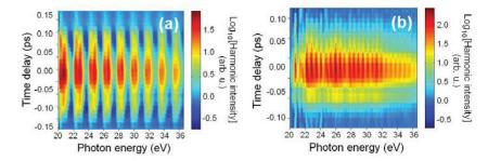
Figure 17. Measured harmonic spectra of argon as a function of delay between  $\lambda_1$ =1300 nm and  $\lambda_2$ = 780 nm pulses, with parallel polarisation (normalised to the harmonic intensity of the 1300 nm field alone). (a)  $I_1$  = 1.5×10<sup>14</sup> W/cm<sup>2</sup>;  $I_2$  = 0.2×10<sup>14</sup> W/cm<sup>2</sup>. (b)  $I_1$  = 0.5×10<sup>14</sup> W/cm<sup>2</sup>.
