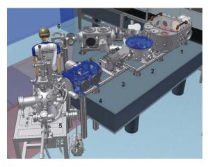
Figure 4. Engineering drawing of the XUV beamlines. Chamber #1 is the XUV generation chamber, #2 is the monochromator, #3 is the flat-field spectrometer (shown in both of its possible locations), #4 are toroidal mirror chambers, #5 is the materials science station and #6 shows the location of the AMO station.
