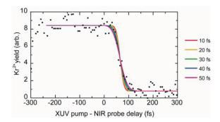
Figure 10. Yield of Kr2+ with harmonic 23 pump and 800nm probe as a function of the delay between the two pulses.
