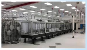
L4 : 10 PW, 130 fs, 2 kJ (PW output, ns uncompressed output)
