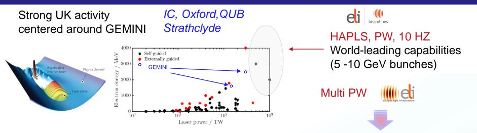
Multi-GeV acceleration in gas cell with f/40 focusing (IC + collaborators)
